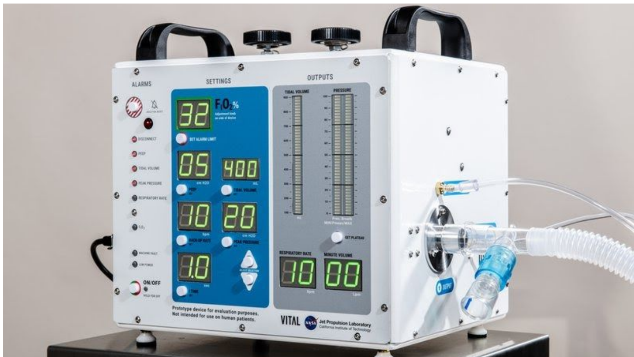
VITAL is a new high-pressure ventilator developed by JPL, tailored to treat coronavirus. Image Credit: NASA/JPL-Caltech
