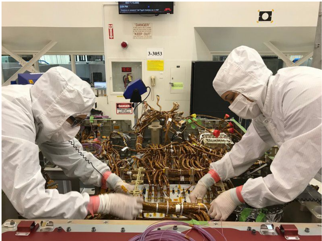
Patricia Lopez (left) Elizabeth Jasso (right) working to install electrical wiring inside the rover. Image Credit: Michael Ilharreguy
