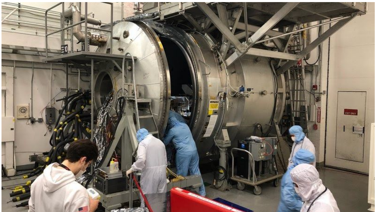
Amila Cooray and the team open the door to the 10-foot horizontal vacuum chamber upon completion of the sterile flight model adaptive caching assembly test. Image Credit: Kenneth Glazebrook
