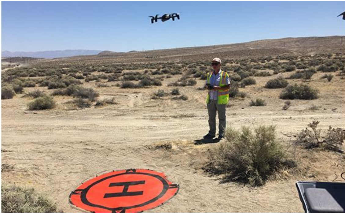
Andrea Donnellan lands drone [small UAS] after flying a grid pattern over the M6.4 rupture south of highway 178 near Trona, California. The vehicle is a Parrot Anafi with a 21 megapixel camera. About 1,500 images are collected per location. (Photos: Erik Conway)
