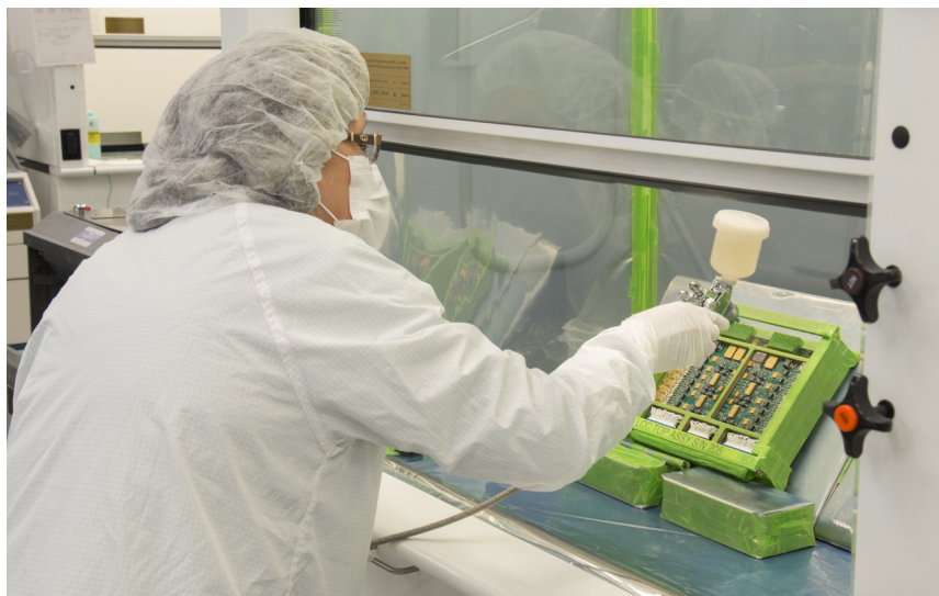
Technician Yolanda Walters works on polymeric conformal coating of an electronics board at the Electronic Fabrication Service Center.
