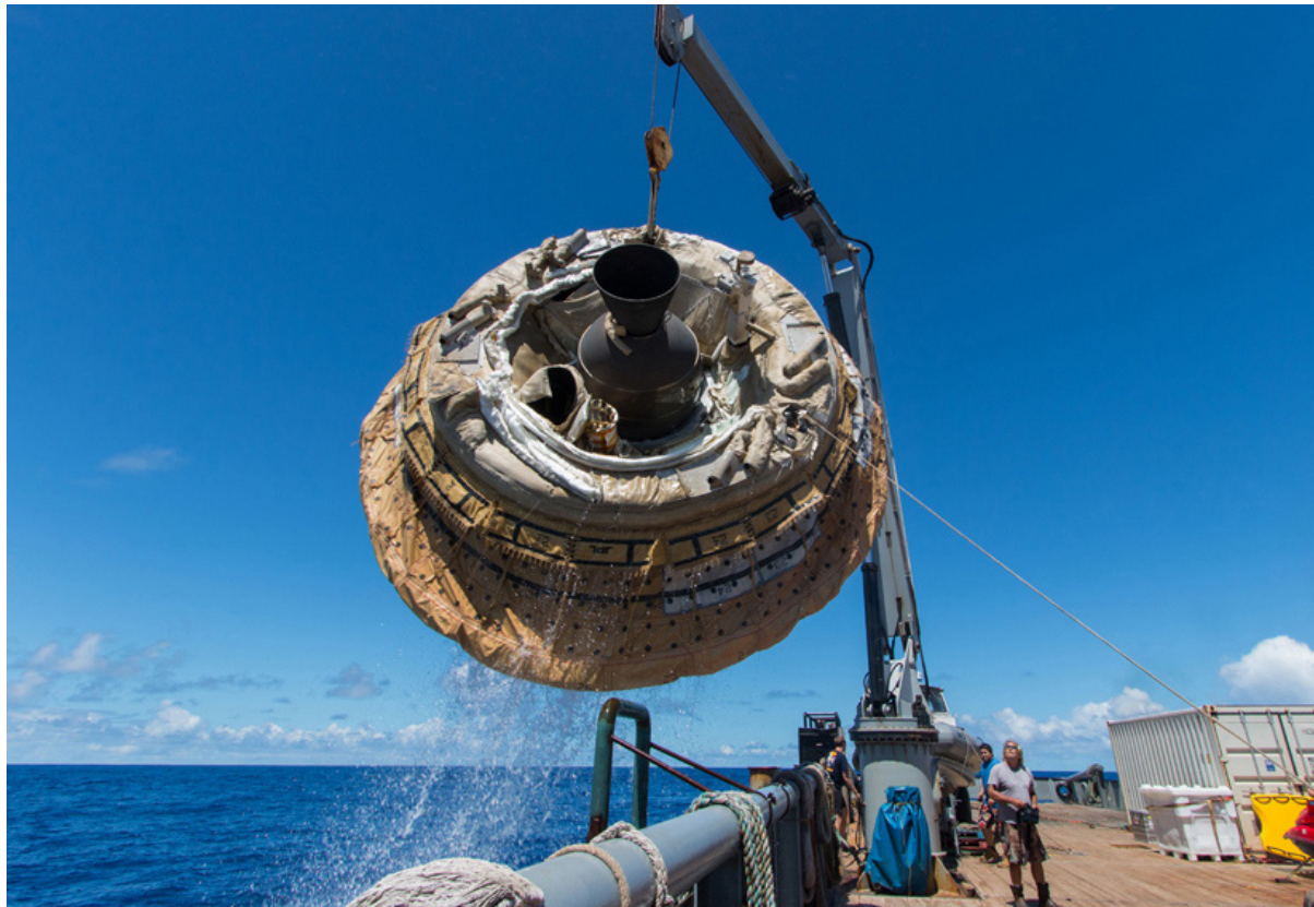
The saucer-shaped Low-Density Supersonic Decelerator test vehicle is lifted aboard the Kahana recovery vessel following the June 28 test off the coast of Kauai.
