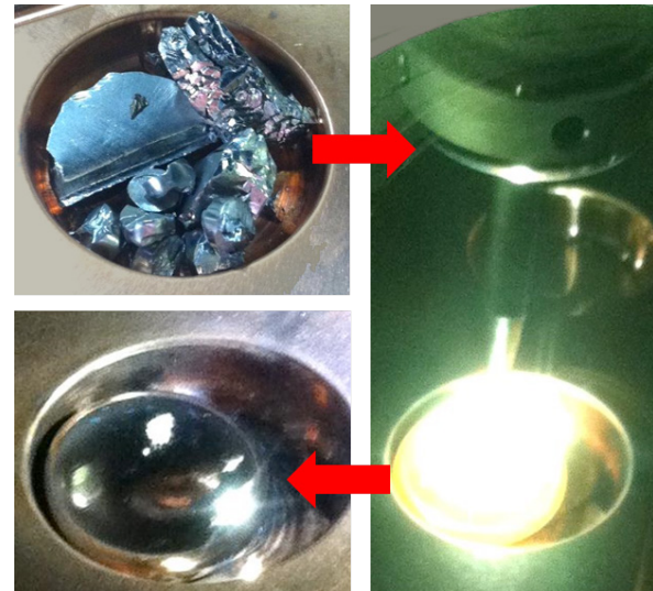
In the arc melter, pure elements are consolidated into homogenous ingots of metal alloys, which are then melted and cast into parts, either for prototyping or for mechanical behavior.
