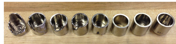
A progression of casting metallic glasses into the shape of a one-inch-diameter hollow cup, which will be later used as a casing for a gearbox.
