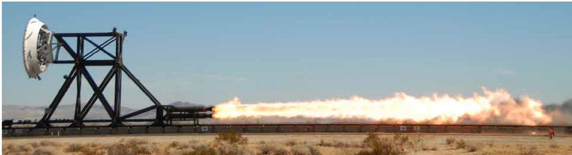
Rocket sled test fixture above replicated the forces a supersonic spacecraft would experience prior to landing. New tests are assessing the Low-Density Supersonic Decelerator Project.
