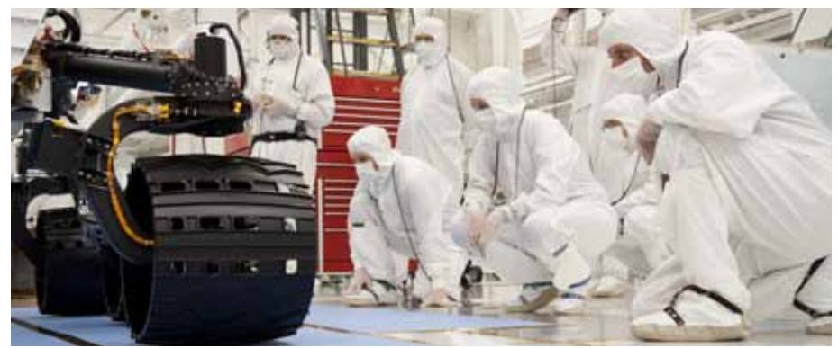
Technicians and engineers in the Spacecraft Assembly Facility survey Mars Science Laboratory's Curiosity rover as it goes for its first test drive July 22.
