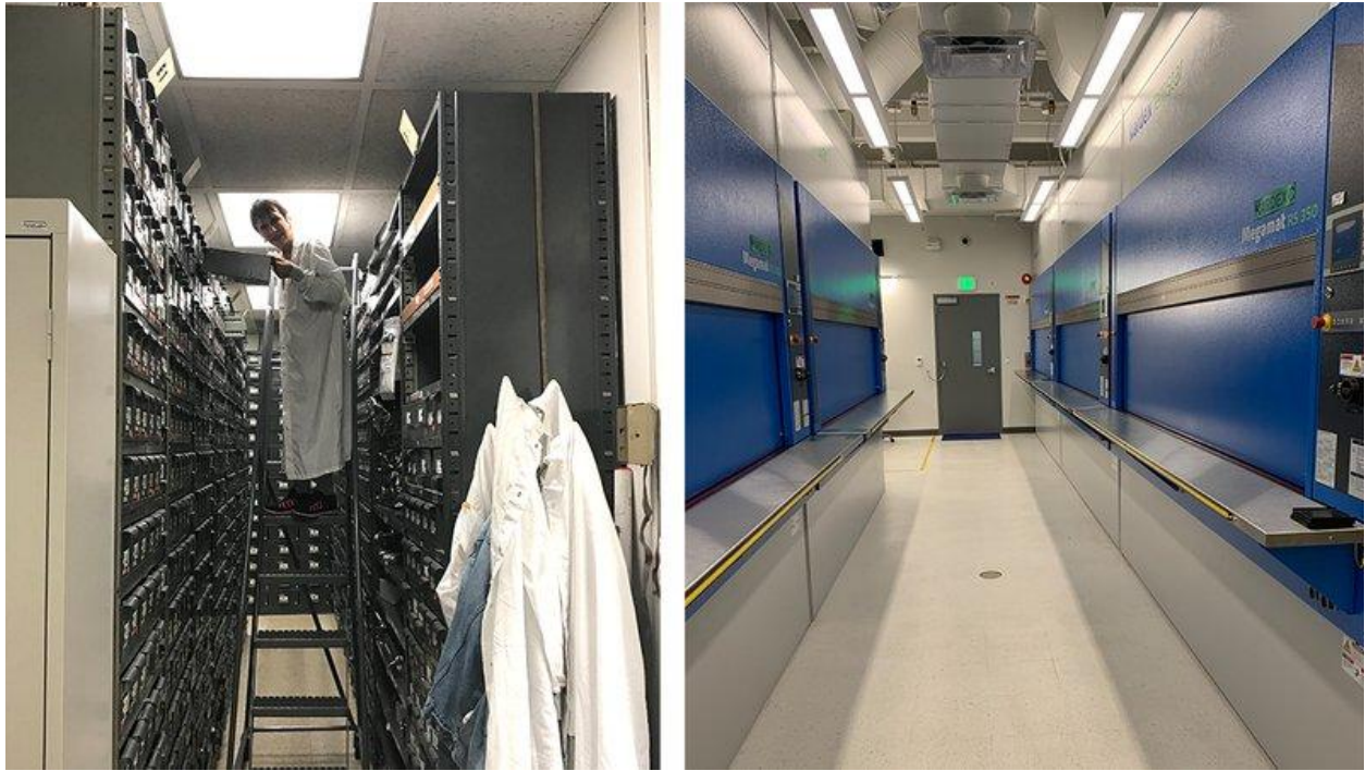
Left: the outdated storage shelving at the old "Flight Parts Store." Right: the upgraded Kardex Remstar Megamat carousels that allow for automated parts selection and retrieval.
