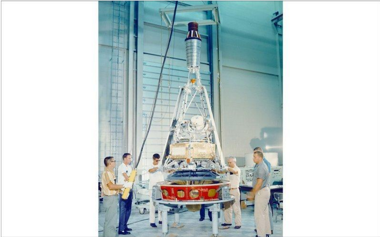
Ranger 1 being mated to its launch vehicle adapter (red ring below the spacecraft), July 5, 1961. Image Credit: NASA/JPL-Caltech
