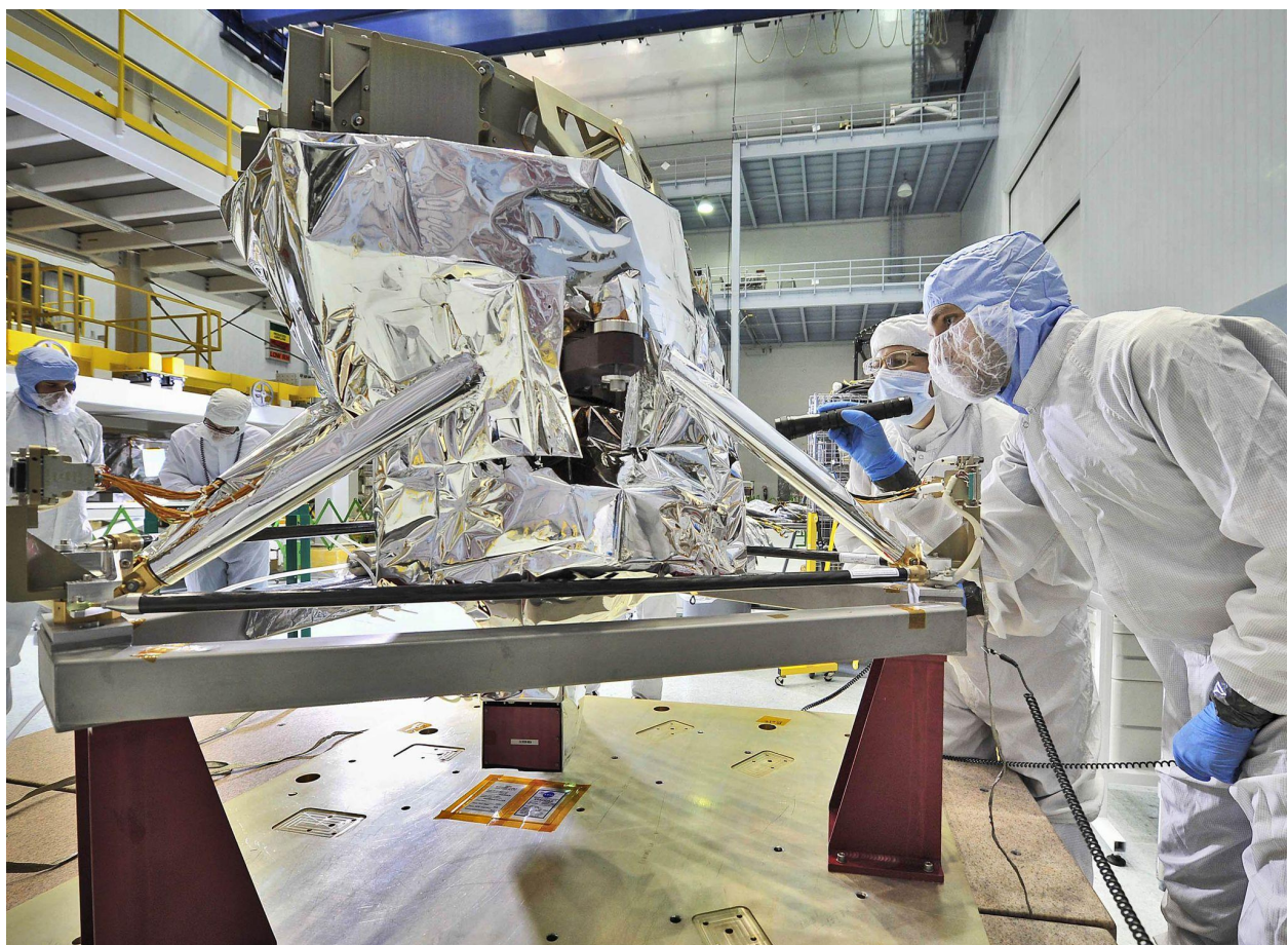
Engineers conduct a "receiving inspection" of the James Webb Space Telescope's Mid-Infrared Instrument. Image Credit: NASA/Chris Gunn.
