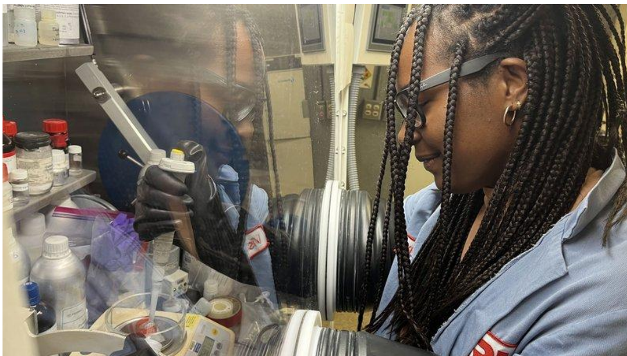
Robinson mixes chemicals to create a battery electrolyte formula for testing.
