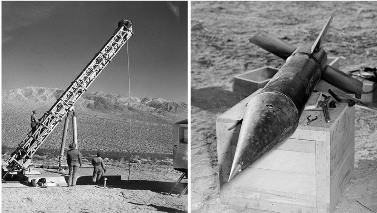
Left: The 32-foot launch tower for the Private missile. Right: The assembled Private missile, weighing in at 500 pounds.
