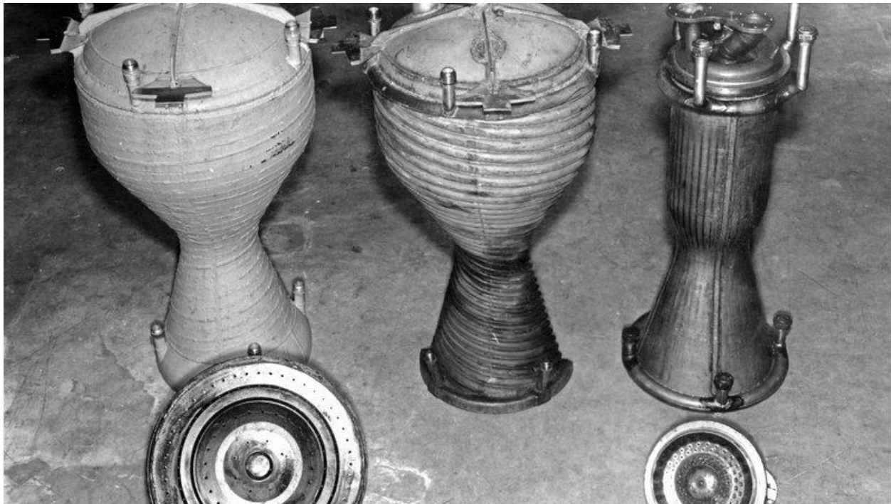
Three generations of Corporal motors. Left to right are the "heavyweight," "lightweight," and "axial cooling" motors. The cooling channel orientation is visible in the surfaces of the motors. The objects in the foreground are the injector plates. Image Credit: JPL/Caltech
