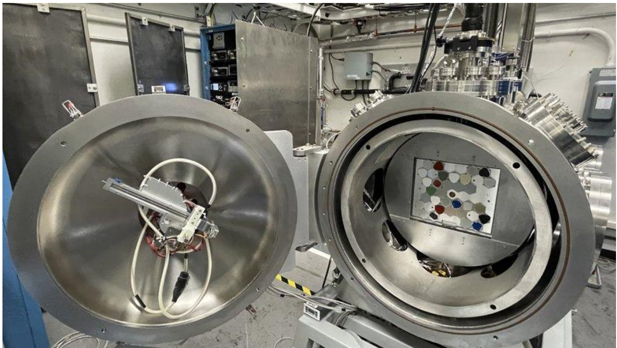
The 90-degree chamber open, showing the sample plate system inside. Image Credit: Courtesy of Nelson Green
