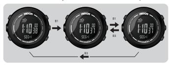
Press B3 to stop the timer. Press & hold B3 again to reset timer to set time.
