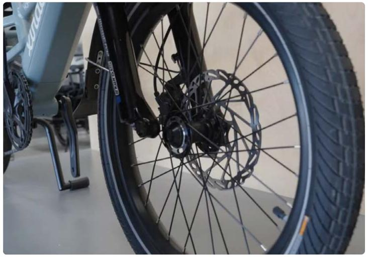
Re-insert the thru-axel, and tighten with a 6 mm hex key.
