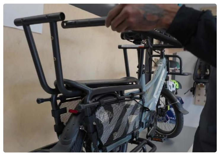
Insert a locking split washer onto each Hooptie rail bolt, and thread into the Hooptie bracket bosses. Tighten with a 4 mm hex key.
