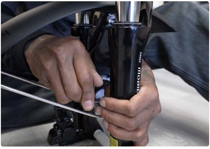
Remove the through axle from the fork with a 6 mm hex key.
