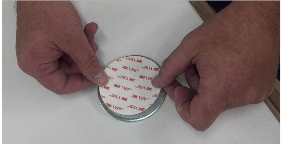
Press the adhesive pad hard against the mounting disk for proper adhesion.
